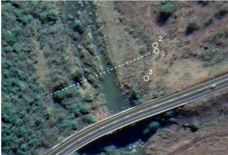
**Figure H3** Location of the surveyed cross-section at the downstream end of a boulder rapid; approximate positions of bench marks/fixed stations are indicated with circular markers; flow direction is top-to-bottom
